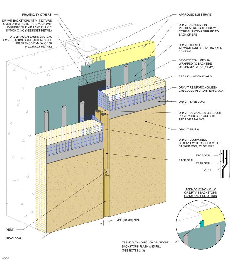
I. DRYVIT RECOMMENDS THAT GROUND FLOOR APPLICATIONS AND ALL FACADES EXPOSED TO ABNORMAL STRESS, HIGH TRAFFIC, OR DELIBERATE IMPACT HAVE THE BASE COAT REINFORCED WITH PANZER® MESH PRIOR TO STANDARD OR STANDARD PLUS MESH. LOCATION OF HIGH IMPACT ZONES SHOULD BE INDICATED ON CONTRACT DRAWINGS.
