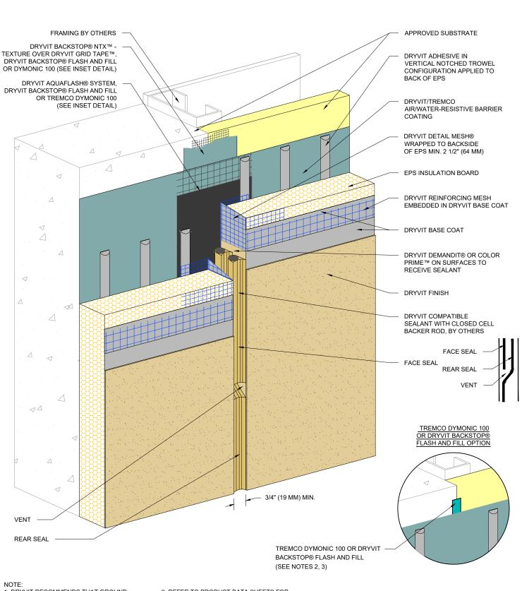
1. DRYVIT RECOMMENDS THAT GROUND FLOOR APPLICATIONS AND ALL FACADES EXPOSED TO ABNORMAL STRESS, HIGH TRAFFIC, OR DELIBERATE IMPACT HAVE THE BASE COAT REINFORCED WITH PANZER® MESH PRIOR TO STANDARD OR STANDARD PLUS MESH. LOCATION OF HIGH IMPACT ZONES SHOULD BE INDICATED ON CONTRACT DRAWINGS.
