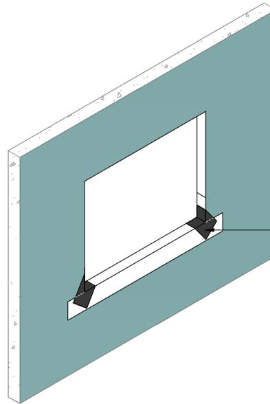
INSTALL DIAGONAL STRIP OF DRYVIT AQUAFLASH® MESH AND AQUAFLASH® SYSTEM AT CORNERS (SEE NOTES 1 AND 3)
