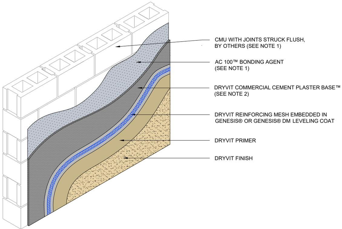
**MASONRY SUBSTRATE WITH DRYVIT BASE COAT
