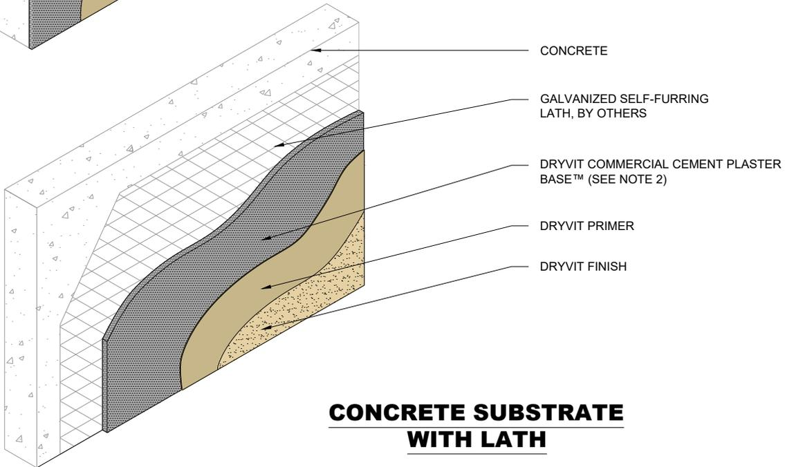
**CONCRETE SUBSTRATE WITH LATH**
