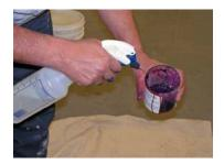
If needed, add untinted finish to the Tint Pack, replace lid, shake vigorously and empty contents into center of finish.
