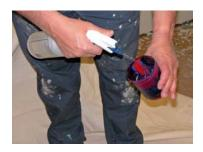
Using a spray bottle, use a small amount of water (no more than 4 fluid ounces total per Pack, per 5 gallons of finish) to rinse out the colorant.
