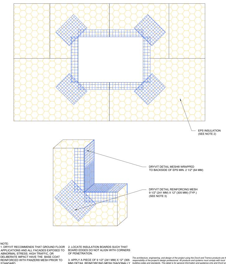
OR STANDARD PLUS MESH. LOCATION OF HIGH IMPACT ZONES SHOULD BE INDICATED ON CONTRACT DRAWINGS.
