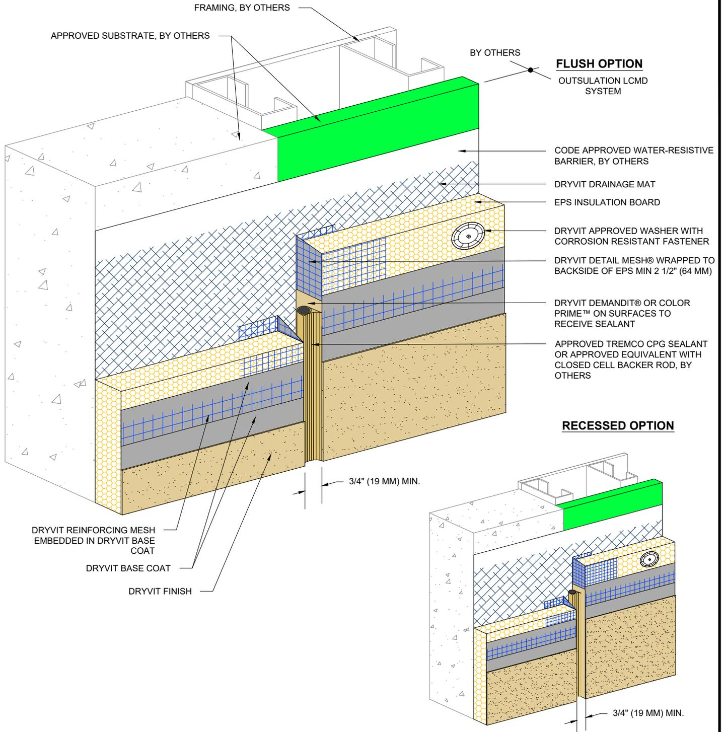
DRYVIT REINFORCING MESH EMBEDDED IN DRYVIT BASE COAT
