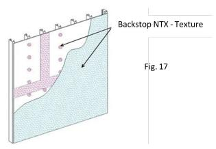
4) The Backstop NTX - Texture material should be applied in a uniform, continuous film at the recommended coverage rate. **NOTE: Substrates with a surface texture or high porosity will require additional material.**
