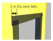
6) Install diagonal "butterflies" consisting of AquaFlash Liquid and AquaFlash Mesh at each sill/jamb corner – Figure
