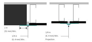
c. Using a brush or 3/4 in (19 mm) nap roller, apply a liberal coat of AquaFlash Liquid material to the backer rod and adjacent substrate surface to the width of the AquaFlash Mesh - Figure 15.
