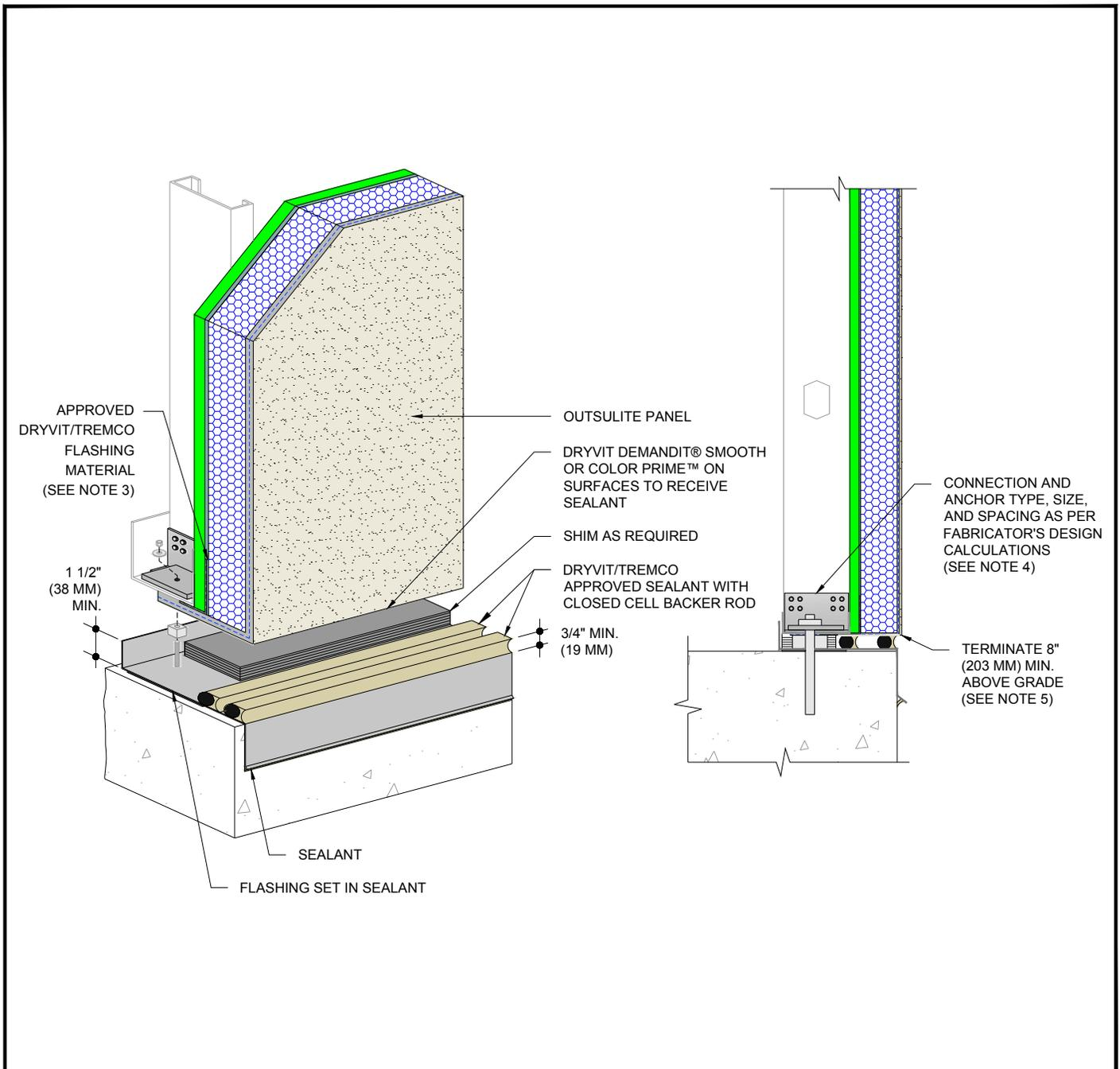
Termination at Slab on Grade<sup>4</sup>
