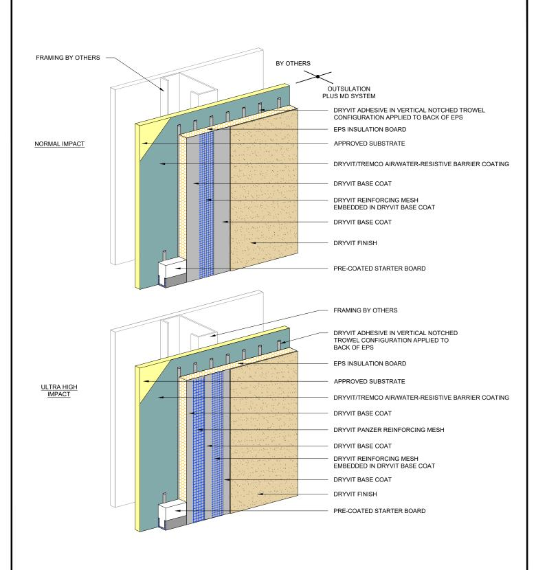
1. DRYVIT RECOMMENDS THAT GROUND FLOOR APPLICATIONS AND ALL FACADES EXPOSED TO ABNORMAL STRESS, HIGH TRAFFIC, OR DELIBERATE IMPACT HAVE THE BASE COAT REINFORCED WITH PANZER® MESH PRIOR TO STANDARD OR STANDARD PLUS MESH, LOCATION OF HIGH IMPACT ZONES SHOULD BE INDICATED ON CONTRACT DRAWINGS.
