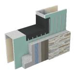
Dryvitoffersafamilyofperformance-basedsystems that allows architects andownersto meetthespecificdemandsof today's energy codes, such ascontinuous insulationand anair/water-resistive barrier.Dryvit's originalOutsulation Systemhasbeen installedonover 500,000 buildings worldwide. Duetothe increaseddemandsfora wall system tobeableto drain away incidental moisture, the Outsulation concepthasgrown intoafamily of related systems, eachbuildingupon the othertoachieve specificperformancegoals.
