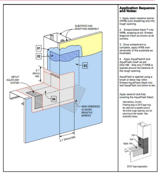
Figure 2: Protection of Rough Openings
