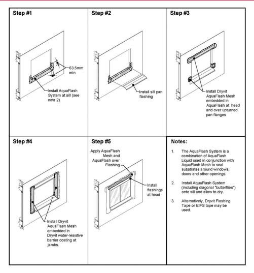
Figure 3: Rough opening and sill preparation – AquaFlash System
